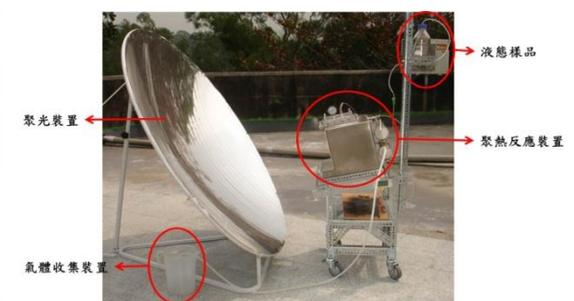
Solar heat for pyrolysis of biomass.
