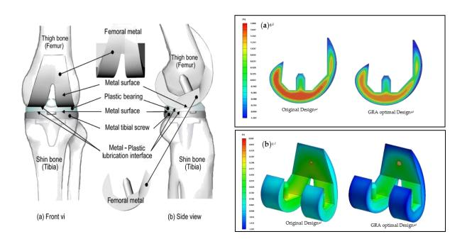
TOPIC: Hybrid Taguchi–Gray Relation Analysis Method for Design of Metal Powder Injection Molded Artificial Knee Joints with Optimal Powder Concentration and Volume Shrinkage
