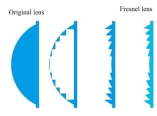
Fig. 1 Fresnel lens shaping process (from left to right)
