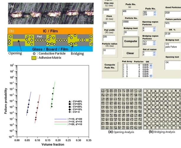
TOPIC: Random dispersion effects of conductive particles on anisotropic conductive film's (ACF's) bonding yield
