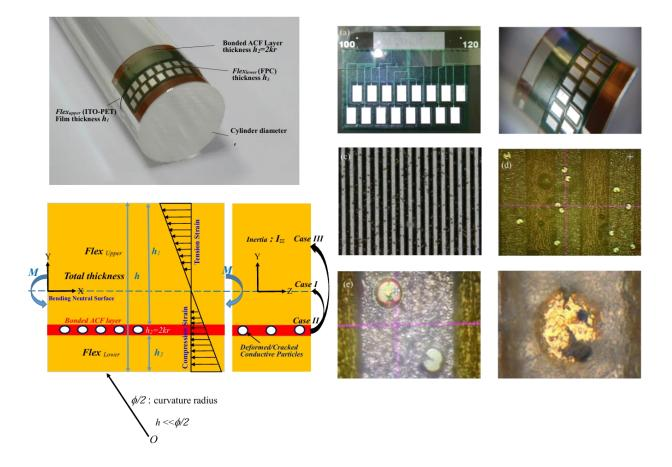
TOPIC: Effects of Bonding Position on Bending Behavior of Flexible Anisotropic Conductive Film Packages considering Neutral Surface
