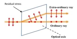
Fig. 2 Effect of residual stress in inducing birefringence in transparent materials
